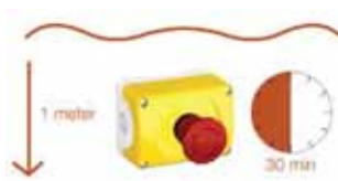
IP67: Submersion to one meter for 30 minutes
